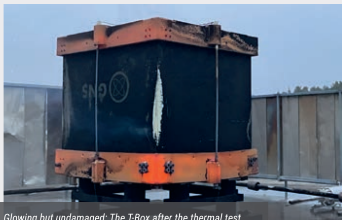
Glowing but undamaged: The T-Box after the thermal test.
