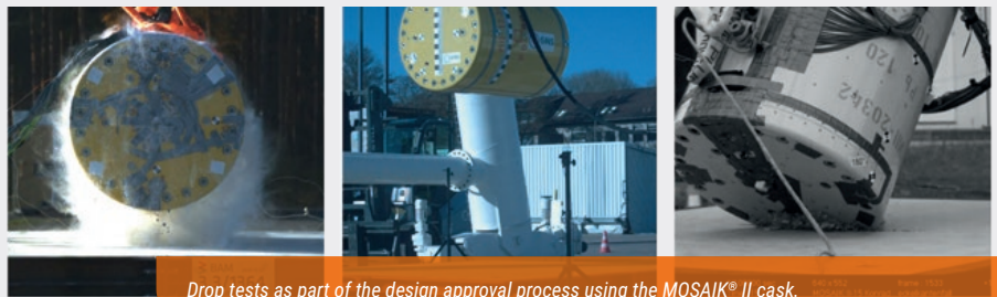
Drop tests as part of the design approval process using the MOSAIK® II cask.
