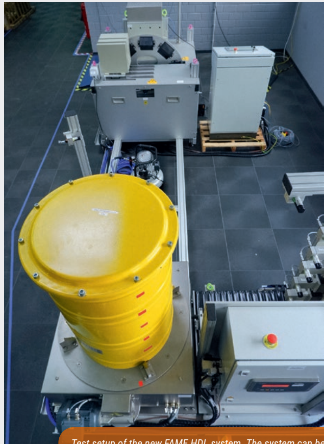
Test setup of the new FAME HDL system. The system can be installed on a footprint of approximately 19 m 2 .
