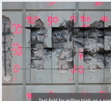
Test field for milling trials on a concrete wall using the newly developed milling method.
