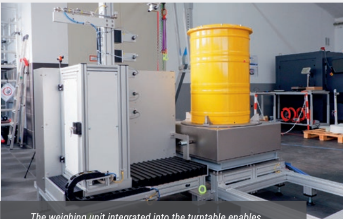
The weighing unit integrated into the turntable enables determination of the drum weight.
