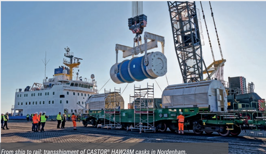
From ship to rail: transshipment of CASTOR® HAW28M casks in Nordenham.
