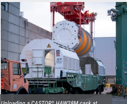
Unloading a CASTOR® HAW28M cask at the Philippsburg interim storage facility.
