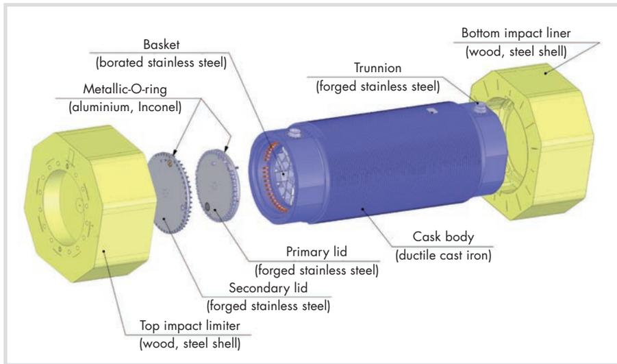
Fig. 3. CASTOR® V/19 in transport configuration (with impact limiters).
