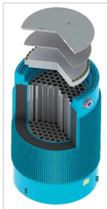
Fig. 8. Schematic diagram of a CONSTOR® cask for hexagonal fuel assemblies.
