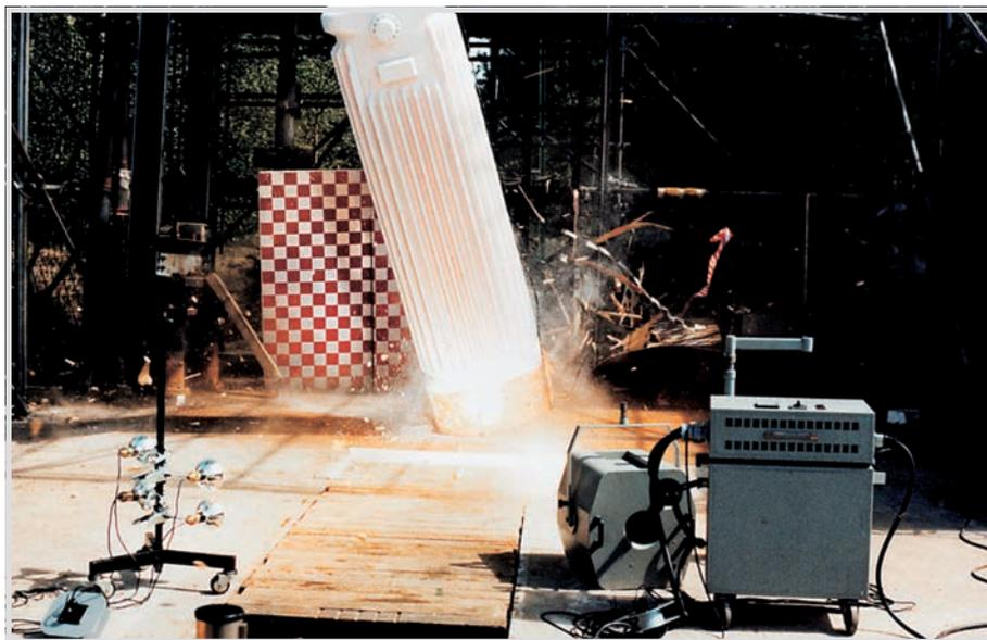
Fig. 2. Drop test of CASTOR® IA.
