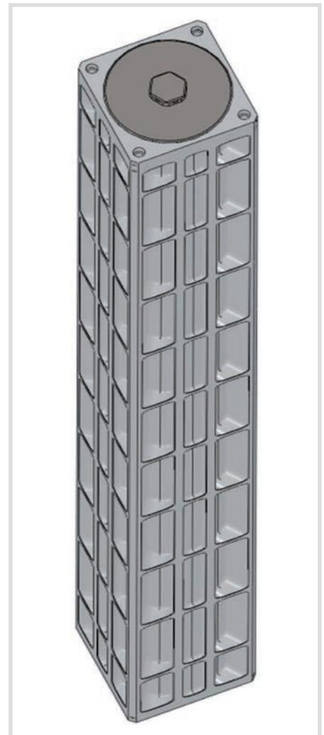
Fig. 9. Quiver for special fuel rods (schematic illustration).
