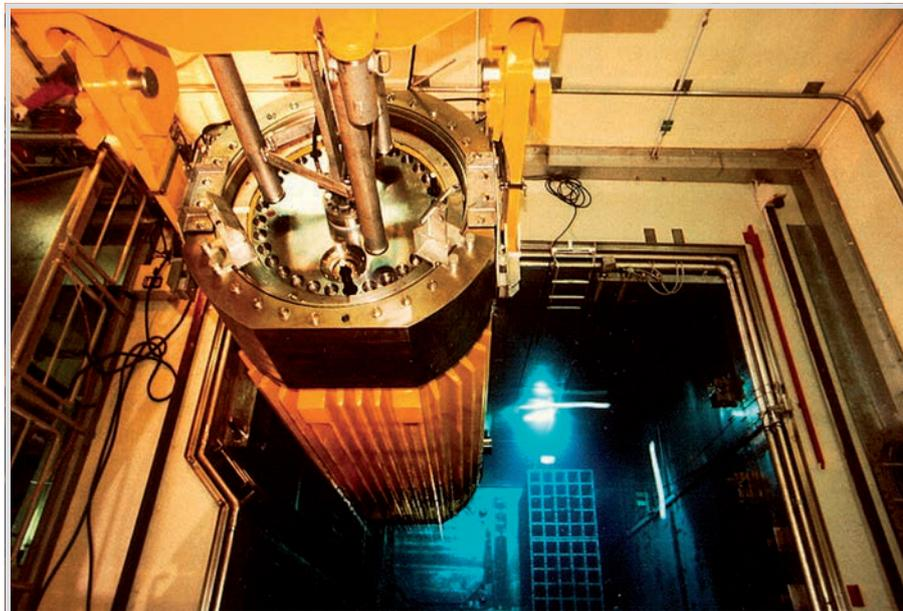
Fig. 4. CASTOR® Ib after loading.
