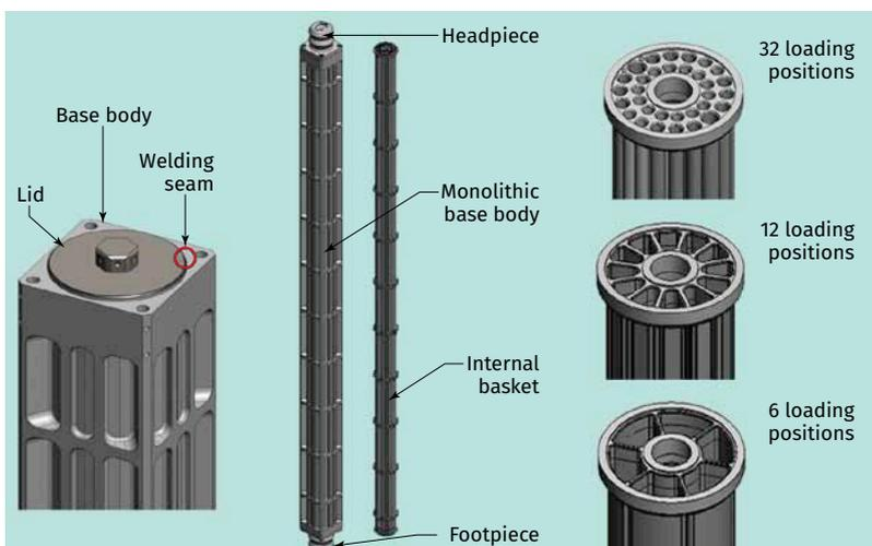
Figure 1: PWR-Quiver for damaged fuel rods: Sealing system (left), head- and foot piece mounted to the base body and internal basket (middle) and example configurations of internal baskets (right)
