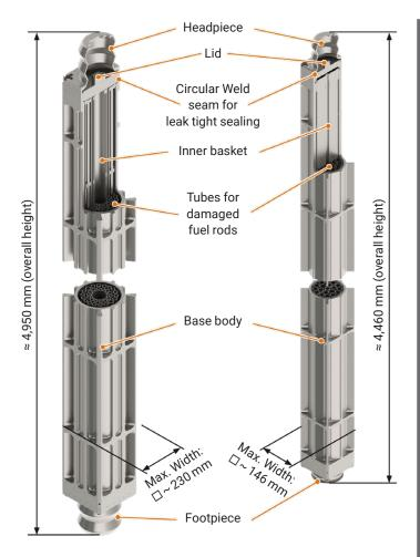
Quiver for casks for Pressurized Water Reactors
